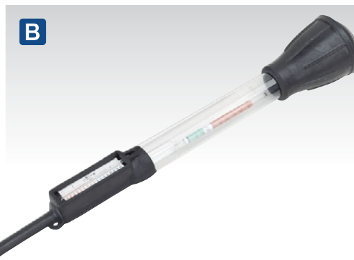
B AK414 6/12/24V Battery Fluid Tester - Tube Type Professional battery hydrometer. Tests 6, 12 and 24V batteries. Float gauge and thermometer built-in. Tube construction with thermometer for temperature compensation.
