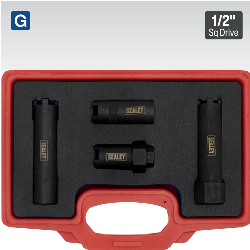
G VS2061 4pc Injector Socket Set - Commercial Suitable for the removal and installation of truck and bus diesel injectors. Castellated socket fits common injectors on MAN, Mercedes, Neoplan and Setra. Also suitable for some Iveco, Renault and Scania vehicles. Supplied in storage case.
