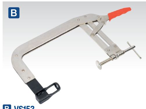
B VS153 OHC/OHV/CVH Valve Spring Compressor Suitable for most small and medium sized OHC engines and also for general use on OHV and CVH engines. Universal jaw with 60-155mm capacity and 160mm throat depth. Parallel lift action with automatic lock.
