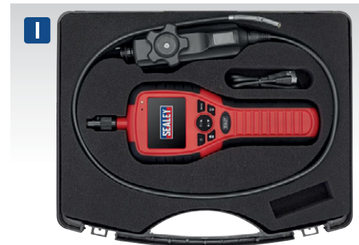
I VS8233A Ø6mm Video Borescope - Articulated Portable articulated borescope supplied with 70mm TFT colour display. Mini waterproof (IP67) camera with integral light (Ø6mm) mounted on 800mm flexible 2-way articulated probe. Using an attached dial, the camera head angle can be changed by up to 350° without having to remove camera from inspection area. Using 8GB micro SD card (supplied) up to 9hrs of video and 20000 still images can be recorded. Videos and still images can be downloaded to a PC via USB data cable (supplied). CMOS camera with six LED probe light and a focus distance of 20-50mm for fine control of light output and clear pictures. Potential applications; automobile maintenance, engine inspection, pipe line exploration etc. Powered by 4 x AA batteries (not included). Camera Probe Length: 800mm Camera: Ø6mm Mirror Flip/Rotate Function: ✓ Pod Length: 20mm Power Source: 4 x AA Batteries (not included)
