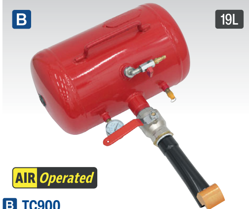
B TC900 19L Bead Seating Tool - Lever Trigger The easy and instant way to seat tubeless tyre beads. Dumps air into tyre void forcing bead to seat against rim for inflation. Air release is controlled by a hand lever operating a ball valve. Fully certified tank with gauge and safety valve prevents over pressurising. Suitable for use on cars, commercials, agricultural and ATV tyres.
