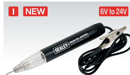
I AK5000 6-24V Circuit Tester Suitable for 6-24V DC circuits. Insulated body with test light. Probe tip is covered with protective plastic cap. Tester illuminates when voltage is present. Supplied with cable and alligator earth clip.
