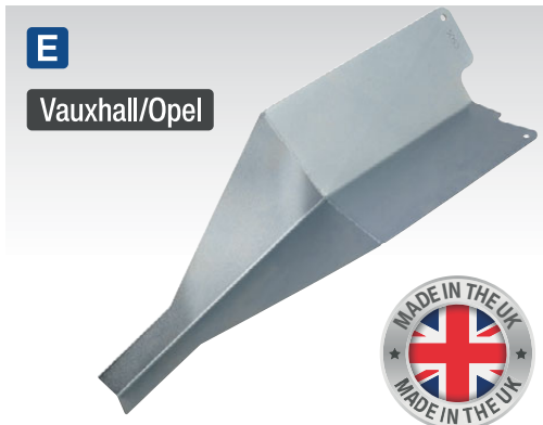
E VS5053 Oil Filter Drain Funnel - Vauxhall/Opel Designed to reduce the amount of time taken to replace the engine oil filter on Vauxhall/Opel vehicles fitted with the B20 diesel engine. Once the drain funnel is located, oil draining from the oil filter can be channelled into a suitable receptacle. Time-saving tool as it eliminates oil spillage onto vehicle chassis and components during filter change.
