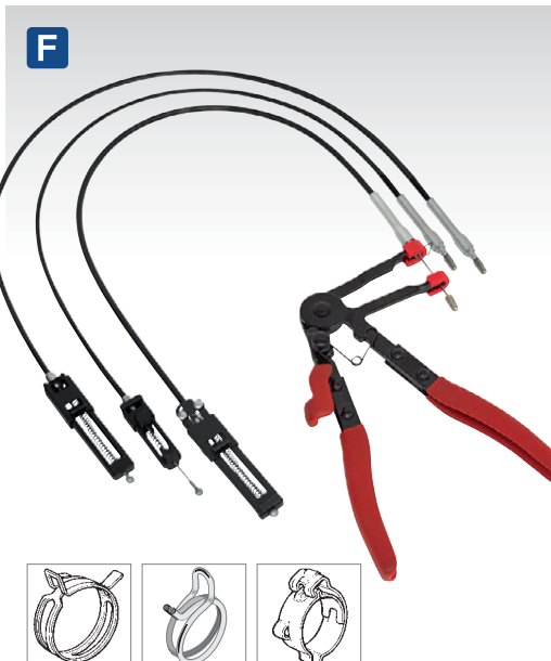
E VS1670 Heavy-Duty Remote Action Hose Clip Tool Reinforced long reach tool designed to get to awkwardly positioned tag-type hose clips. Flexible cable and compact head help operation in confined spaces. Features ratchet action for close control.
