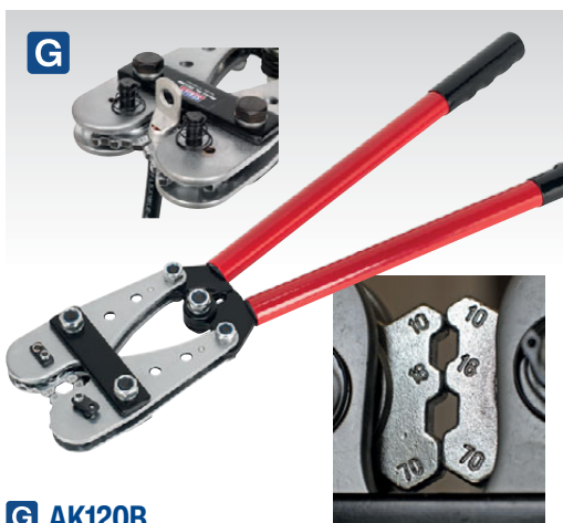
G AK120B 10-120mm 2 Copper Lug Terminal Crimping Tool Range is 10-120mm 2 . BS Standard type terminal. Manufactured from SCM-40 hard tool steel. Accurate bore diameter and good crimping effect.
