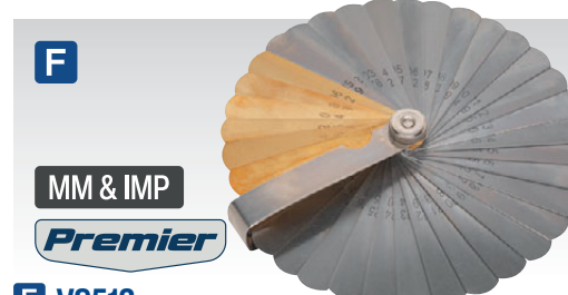
F VS513 36 Blade Combination Steel/Brass Feeler Gauge - Dual Marked 30 Steel blades and six brass blades for non-magnetic applications on electronic ignition systems. Blade dimensions 75 x 13mm. Blade Sizes: Imperial Steel: 0.002", 0.0025", 0.003", 0.004", 0.005", 0.006", 0.007", 0.008", 0.009", 0.010", 0.011", 0.012", 0.013", 0.014", 0.015", 0.016", 0.017", 0.018", 0.019", 0.020", 0.021", 0.022", 0.023", 0.024", 0.025", 0.026", 0.028", 0.030", 0.032", 0.035" Imperial Brass: 0.006", 0.008", 0.010", 0.012", 0.014", 0.016" Metric Steel: 0.051, 0.063, 0.076, 0.102, 0.127, 0.152, 0.178, 0.203, 0.229, 0.254, 0.279, 0.305, 0.330, 0.356, 0.381, 0.406, 0.432, 0.457, 0.483, 0.508, 0.533, 0.559, 0.584, 0.610, 0.635, 0.660, 0.711, 0.762, 0.813, 0.889mm Metric Brass: 0.152, 0.203, 0.254, 0.305, 0.356, 0.406mm
