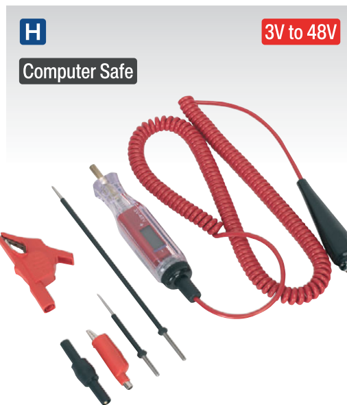
H PP5 3-48V Integrated Test Light/Voltmeter LCD meter draws minute currents making this tool safe to use around delicate electronic components. With a range of 3-48V DC, this tool is suitable for motorcycle, car and commercial applications. Includes interchangeable 65 and 175mm probes, leads and clips with Ø4mm banana coupling.
