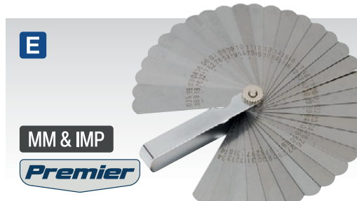
E VS512 35 Blade Feeler Gauge - Dual Marked Blade dimensions 75 x 13mm. Blade Sizes: Imperial: 0.0015", 0.002", 0.003", 0.004", 0.005", 0.006", 0.007", 0.008", 0.009", 0.010", 0.011", 0.012", 0.013", 0.014", 0.015", 0.016", 0.017", 0.018", 0.019", 0.020", 0.021", 0.022", 0.023", 0.024", 0.025", 0.026", 0.027", 0.028", 0.029", 0.030", 0.031", 0.032", 0.033", 0.034", 0.035" Metric: 0.038, 0.051, 0.076, 0.102, 0.127, 0.152, 0.178, 0.203, 0.229, 0.254, 0.279, 0.305, 0.330, 0.356, 0.381, 0.406, 0.432, 0.457, 0.483, 0.508, 0.533, 0.559, 0.584, 0.610, 0.635, 0.660, 0.686, 0.711, 0.737, 0.762, 0.787, 0.813, 0.838, 0.864, 0.889mm
