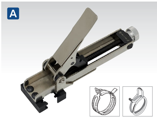
A VS1575 Spring Hose Clip Tensioner Tool Locks in place for safe clip removal/refitting. Ideal for use in confined areas. Single-handed use. Range 5-55mm.
