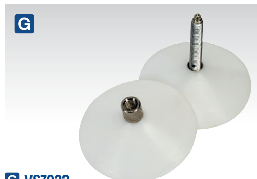
G VS7022 Universal Bearing Packer Suitable for packing bearings with an even spread of grease. Clean, quick operation simply place bearing on to the bottom cone, screw down the cone lid and pump grease into nipple. Works on most tapered roller bearings fitted on cars, boats, trailers, etc. Both cones feature knurled grips for use with oily fingers. Suitable for use with Sealey and other best-selling grease guns. Maximum Cone Diameter: Ø104mm Shaft (Height x Diameter): 60 x Ø11mm
