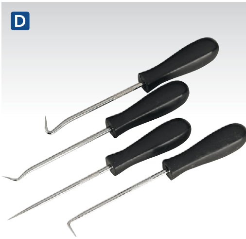
D AK521 4pc Mini Hook Set Chrome finish shafts with knurling for fingertip precision. Suitable for removal of bushings, cotter pins, O-rings and seals. Classic styled handles. Contents: Straight, Right Angle, Half-Round, Swan Neck Length: 125mm
