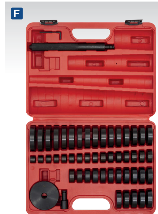
F VS7032 52pc Bearing Race & Seal Driver Set Set of 49 square edged heavy-duty steel drivers from Ø18mm to Ø74mm. Suitable for installation of bearings or seals without damaging the bearing, seal or housing. Adaptors can also be used in a standard workshop press. Supplied in storage case.
