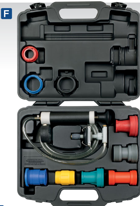
Kit includes cap test adaptors - simply insert bladder into adaptor and inflate.
