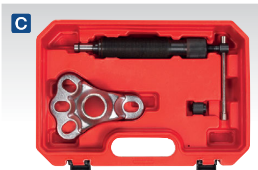
C PS993 10 Tonne Hydraulic Hub Puller Set Puller yoke with 10 Tonne hydraulic ram. Suitable for four and five stud hubs. Hydraulic ram provides additional power to extract the most stubborn hubs. Minimum/Maximum Stud Spread: 85/128mm Maximum Hub Flange: 64mm 4-Stud Min./Max. Hole Spacing: 84 -127mm 5-Stud Min./Max. Hole Spacing: 79 -122mm
