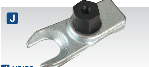
J VS150 CVH Valve Spring Compressor - Ford Permits valve stem seal and valve spring replacement without the need to remove the cylinder head. Superior cast design with radiused fulcrum for smooth spring compression. Suitable for CVH Ford engines 1.3, 1.4 and 1.6 as fitted to Escort (inc. XR3i and RS Turbo) and Fiesta (inc. RS Turbo).
