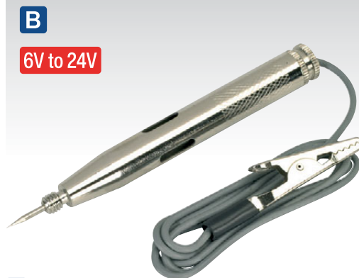
B AK4008 6-24V Circuit Tester Suitable for 6-24V DC circuits. Knurled brass body with test light. Probe tip is covered with protective brass screw cap. Tester illuminates when voltage is present. Supplied with cable and alligator earth clip.
