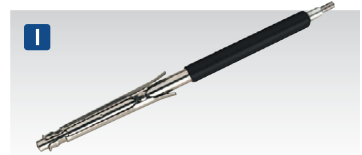
I VS1651 Valve Collet Installer/Remover 8/16/24 Valve Spring loaded shaft and clips aid simple and secure installation of valve spring collets. Quick and easy retrieval of lost collets using magnetic tip. Suitable for 8, 16 and 24 valve engines. Ideal for use on heads with recessed valves.
