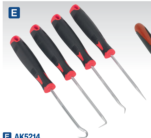
E AK5214 4pc Mini Hook & Pick Set Chrome finish shafts with knurling for fingertip precision. Ergonomically styled handles for comfort, grip and accuracy. Suitable for removal of bushings, cotter pins, O-rings and seals. Contents: Straight, Right Angle, Half-Round, Swan Neck Length: 165mm
