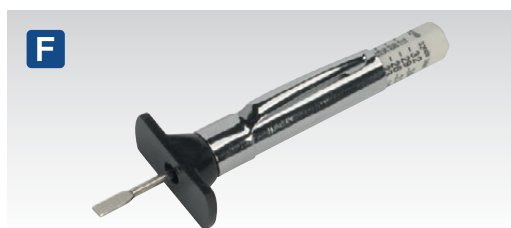
F TST/DGE Tyre Tread Depth Gauge - Pocket Type Chromed steel body with pocket-clip. Scale from 0-25mm in 1mm(0-1" in 1/32") graduations.
