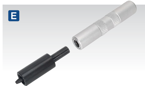
E VS1542 Valve Collet Remover/Installer For quick removal/installation of valve collets, firmly push or tap tool with a hammer, magnet in tool captures collets. Can be used with cylinder head in situ or on workbench. Ideal for replacing broken valve springs or valve stem oil seals without removing the head from the engine. For in situ use, a suitable adaptor (not included) will be required to allow compressed air into the combustion chamber to hold the valve closed while compressing the valve spring.
