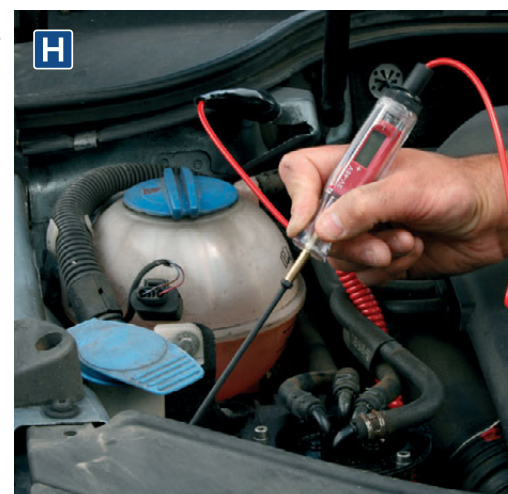
I AK5000 6-24V Circuit Tester Suitable for 6-24V DC circuits. Insulated body with test light. Probe tip is covered with protective plastic cap. Tester illuminates when voltage is present. Supplied with cable and alligator earth clip.
