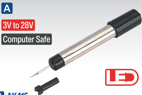
A AK415 3-28V Cordless Circuit Tester Buzzer/LED Suitable for testing DC circuits with voltages between 3 and 28V. No earth clips to get tangled - simply contact the wire to be tested and touch your finger on bare metal ground to get a reading. Tester illuminates LED, buzzes and vibrates on contacting live wire. Computer-safe for use around delicate engine management systems. Supplied fitted with two long-life N-sized batteries.
