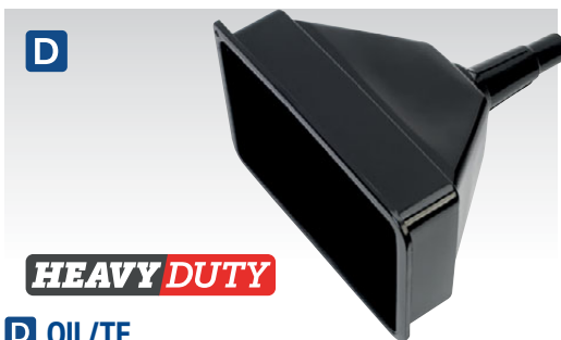
D OIL/TF Tractor Funnel with Debris Filter Heavy-duty funnel manufactured from high-density polyethylene. 255 x 165mm Aperture to accommodate up-ended containers. Supplied with water separating filter. Tapered spout with venting ribs.
