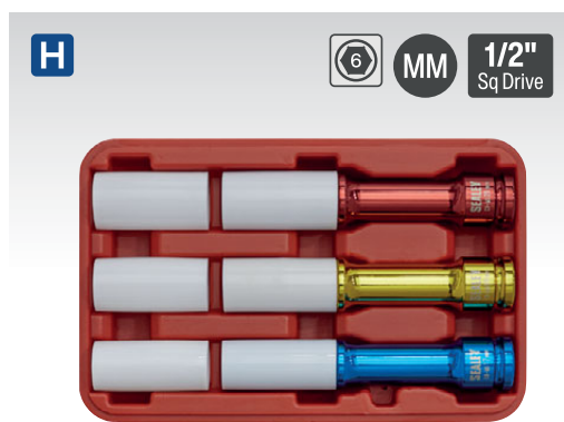
H SX031D 3pc 1/2" Sq Drive Alloy Wheel Long Reach Impact Socket Set Chrome Molybdenum sockets, hardened, tempered and anodised for corrosion resistance. Suitable for use with impact tools. Each 6-point socket is sleeved and has an insert to prevent damage to alloy wheels and nuts. Colour-coded socket assists ease of size selection. Comprises deep or long reach 17, 19 and 21mm sockets. Supplied in storage case.
