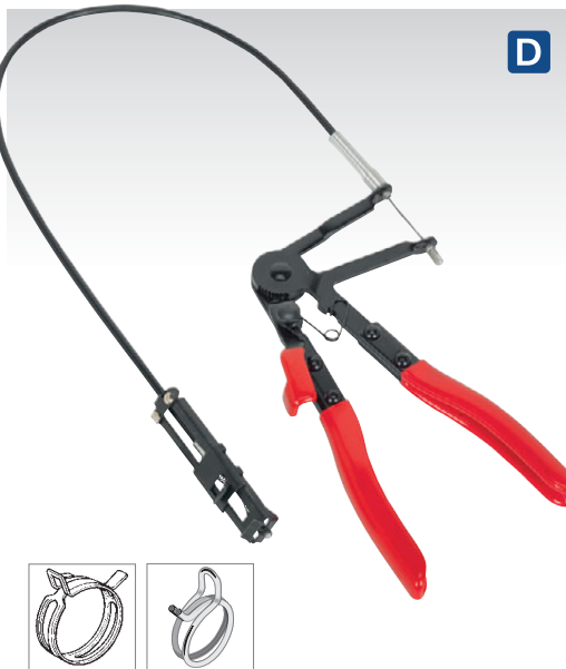
D VS1663 Remote Action Hose Clip Tool Long reach tool designed to get to awkwardly positioned tag-type hose clips. Flexible cable and compact head help operation in confined spaces. Features ratchet action and vinyl dipped handles for comfort and close control.
