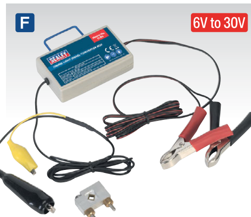
F TL95 Timing Light Diesel Converter Box Used to detect the pulse from the fuel pipes of diesel fuel injectors. Works on most direct injection diesel engines fitted with 6mm(1/4") to 10mm(3/8") external fuel pipes. Suitable for use with most timing lights, engine analysers and multimeters that have an inductive pick-up.
