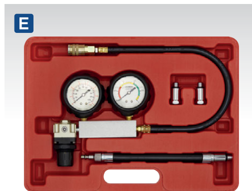
B CT955 8pc Compression Test Kit Compression tester fitted with Ø63mm gauge reading up to 300psi(20kg/cm 2 ). Kit includes 130mm straight and angled push-on connectors, 300mm flexible extension with 10, 12, 14, 18mm adaptors.
