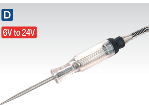
D AK402 6/12/24V Circuit Tester with Test Light Suitable for testing 6, 12 and 24V DC circuits. Insulated, pointed probe tests through wire insulation. Supplied with 1.5m cable and crocodile earth clamp.
