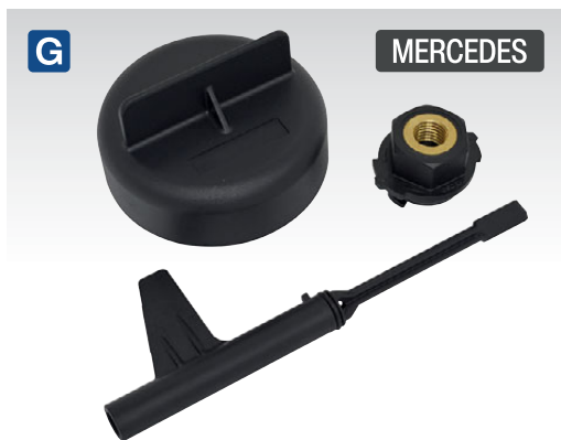
G VS589 Automatic Gearbox Oil Filler Set Mercedes 9G-Tronic Suitable for 9G-Tronic 725 series gearboxes fitted to Mercedes E350 BlueTEC (2013on) and CLS models (2014on). Contains a socket wrench to adjust oil level and a quick release coupling. Designed for drain and refilling operations.
