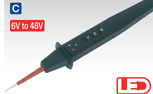
C AK407 6/12/24/48V LED Circuit Tester Suitable for 6, 12, 24 and 48V DC circuits. LED array indicates polarity and voltage range. Supplied with 850mm cable and crocodile earth clamp.
