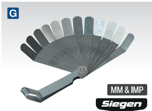
G S0516 12 Blade Offset Feeler Gauge - Dual Marked Imperial and Metric. Offset tips are essential for checking tolerances on OHC configurations and suitable for other applications where straight blades will not fit. Sizes 0.008" to 0.026" (0.203 to 0.660mm). Blade dimensions 95 x 13mm (45°-25mm offset). Blade Sizes: Imperial: 0.008", 0.010", 0.012", 0.013", 0.014", 0.015", 0.016", 0.018", 0.019", 0.020", 0.025", 0.026" Metric: 0.203, 0.254, 0.305, 0.330, 0.356, 0.381, 0.406, 0.457, 0.483, 0.508, 0.635, 0.660mm
